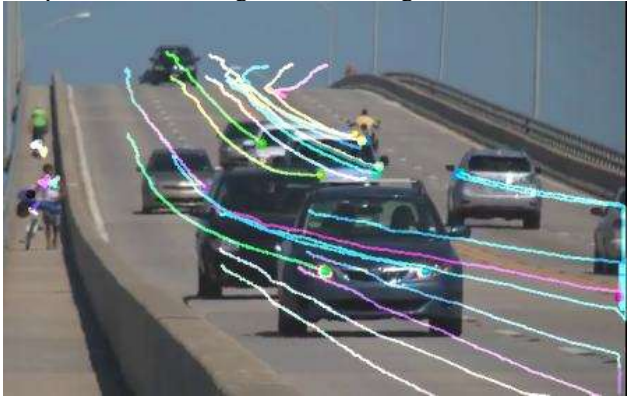
Fig. 4. A demonstration of optical flow. Each coloured line shows where a pixel has moved throughout the video.
