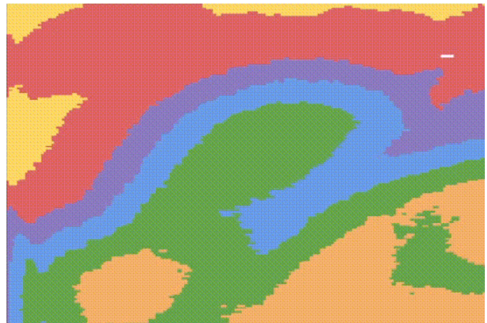
Fig. 12. A section of a different visualisation frame after the 5 frame median & Gaussian blur noise reduction techniques have been applied where the sand has not been moved
