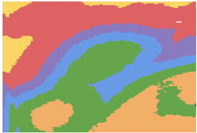
Fig. 11. A section of a visualisation frame after 5 frame median & Gaussian blur noise reduction techniques have been applied
