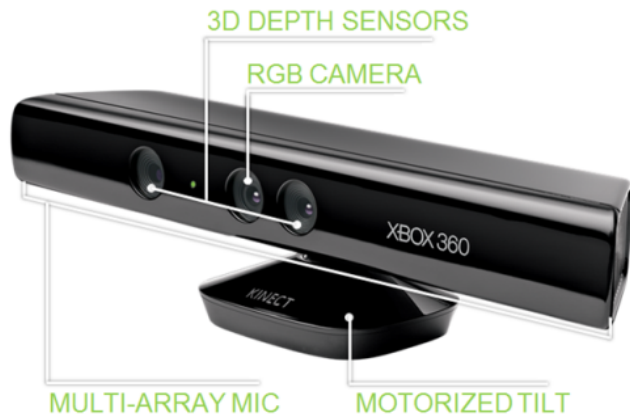
Fig. 2. A diagram detailing the architecture of a Microsoft Kinect for Xbox 360 [11]
