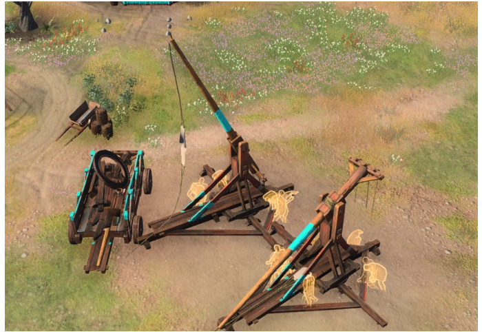
Fig. 1. A traction trebuchet simulation from the game Age of Empires IV. It has thin sticks holding up the axle on either side, which is most likely for aesthetics as it is not practical from an engineering perspective. Source: [5]
