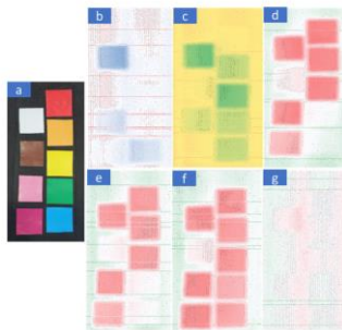
Fig. 5. Spectral data of a color chart for system [7]: (a) image, (b) 405 nm, (c) 532 nm, (d) 650 nm, (e) 740 nm, (f) 850 nm, and (g) 1050 nm.
