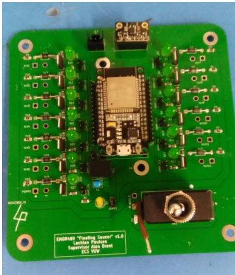
Fig. 16. Final design of the control electronics implemented on a PCB.
