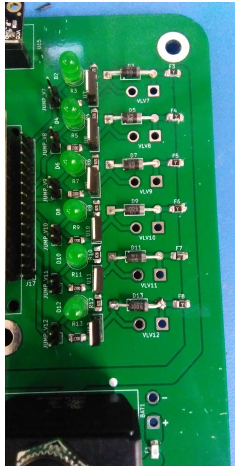
Fig. 15. A column of the completed driver circuit units.
