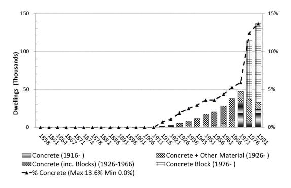
Figure 3: External Wall Concrete Construction 1858 to 1981
