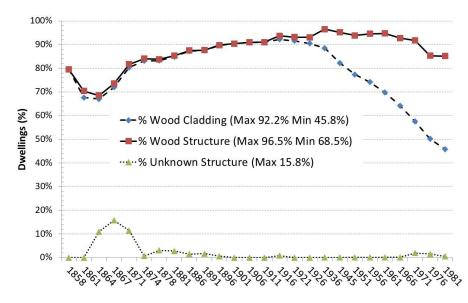
Figure 4: External Wall Cladding and Structure 1858 to 1981
