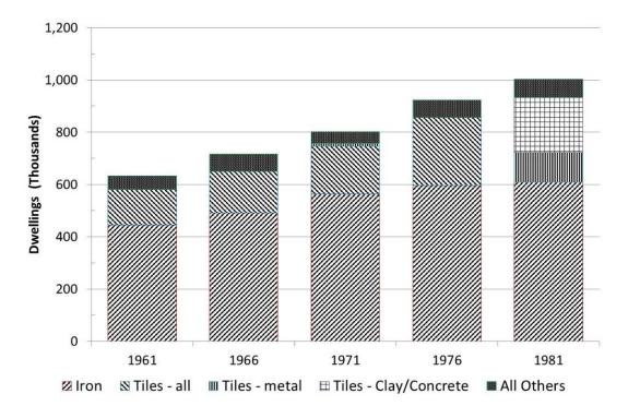
Figure 7: Roof Material Count 1858 to 1981
