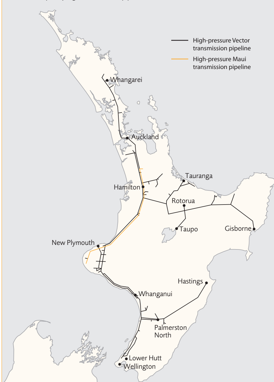
Indicative map: Major gas-transmission pipelines
