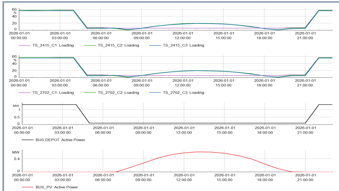
Figure 7. (a) TS_2415 transformer loading in all cases (case1: purple curve, case2: green curve and case3: blue curve) (b) TS_2702 transformer loading in all cases (case1: purple curve, case2: green curve and case3: blue curve) (c) Load profile of the bus depot (d) PV output at the respective time of the day
