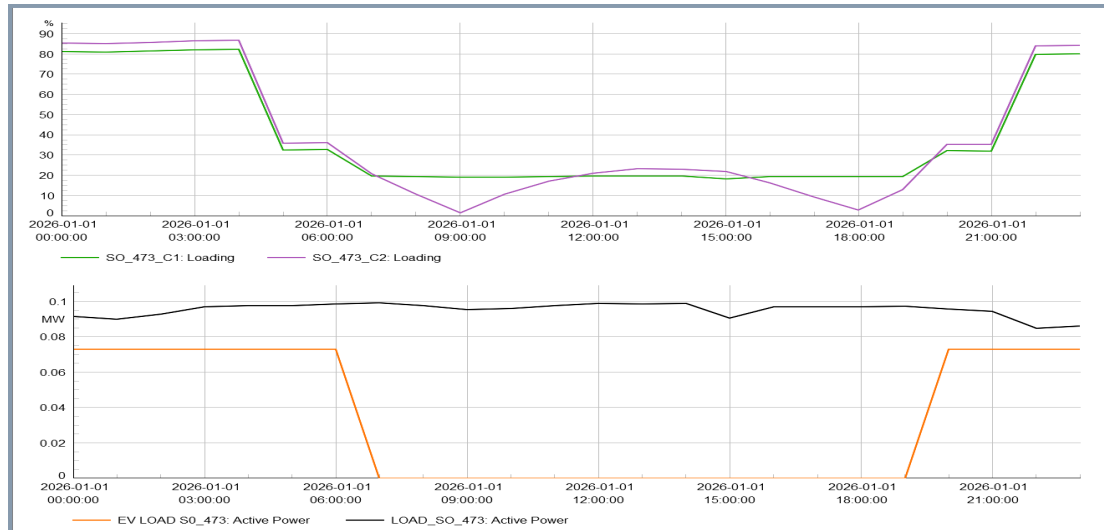
Figure 8. (a) Transformer loading in case 1 (green curve), and case 2 with PV and BESS integration (b) Residential load on the transformer (black curve) and EV loading (orange curve)
