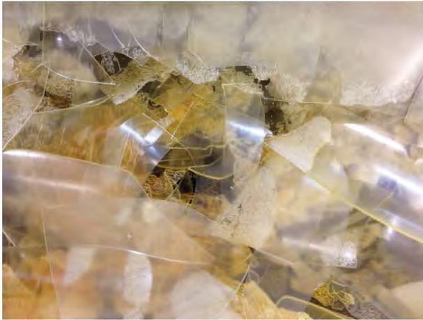
Figure 8: Detail of the degraded Cellulose Nitrate sleeves.
