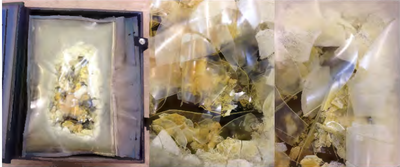
Figure 7: Degraded plastic sleeves.
