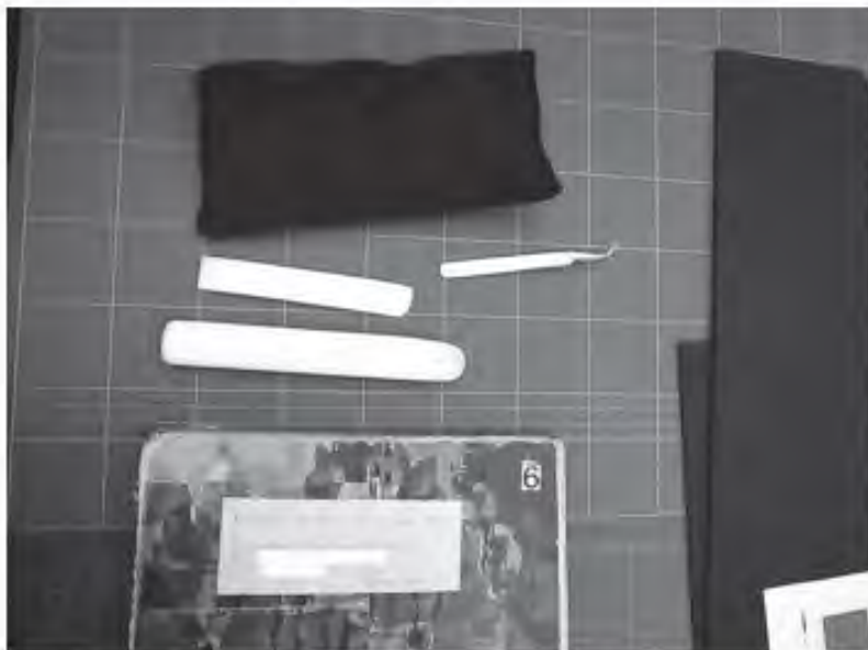
Above – Figure 5: Teflon folder used for lifting sellotape. Photograph by the author, 2015.
